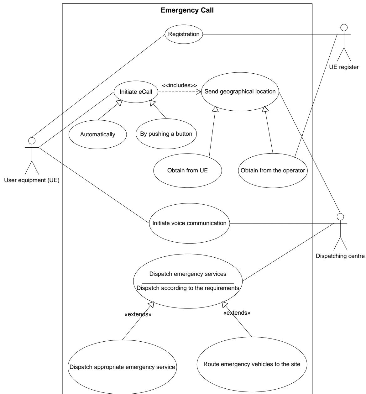
Figure 2: eCall use-case diagram
