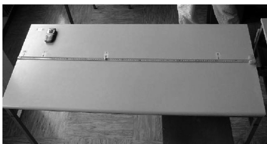
Figure 4: Setup of the experiment with rolling steel balls.
