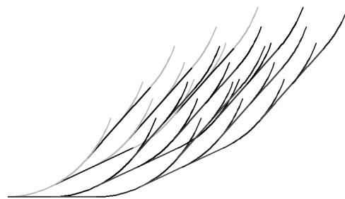
Figure 6. A grammar G_{turn\_left} , for radius R=5m - graphical illustration
