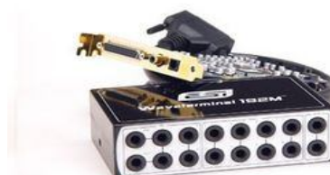
Figure 12.: Waveterminal 192M breakout box and M Appeal sound card (Source: www.proaudio_1892.com/htm1 )
