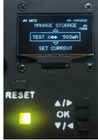
Figure 3. Local user interface used for excitation current selection and manual initiation of the measurement sequence.
