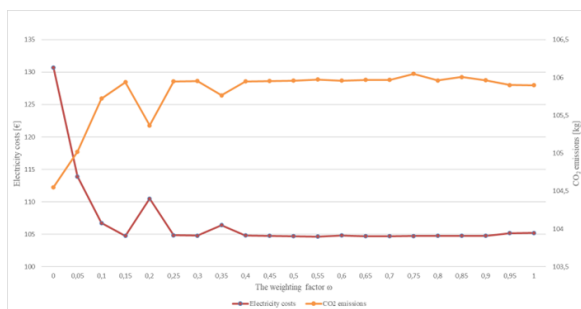
Figure 6. Combined representation of electricity costs and total CO_2 emissions
