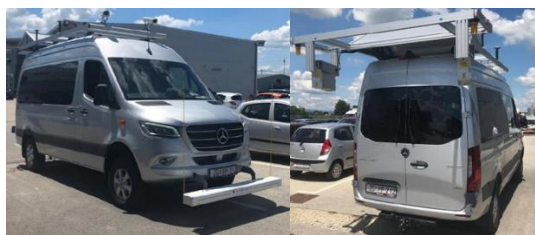
Figure 3. Special vehicle with laser profiler (left) and LCMS system (right)
