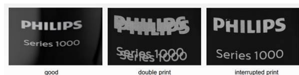
Figure 1: The images considered for this research correspond to well-printed logos (good) or defective prints (double or interrupted prints).
