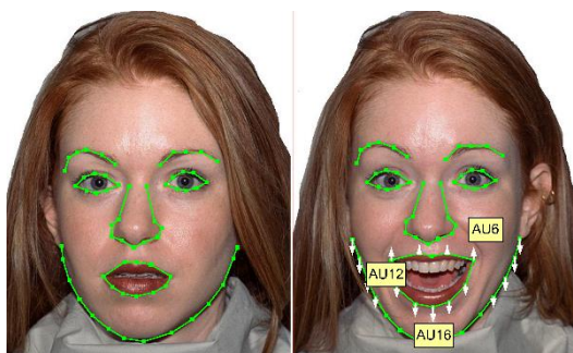
Figure 2. Comparison of spatial features between a neutral face (left) and expression of happiness (right) with affiliated AUs.
