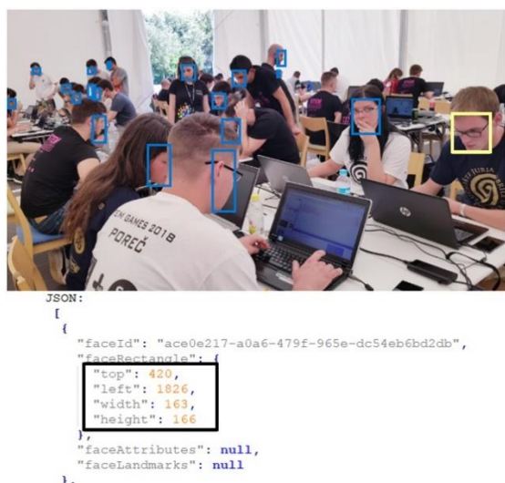
Figure 1. Face detection using Microsoft Cognitive Services API with the accompanying JSON code defining one of the face boxes in the picture.
